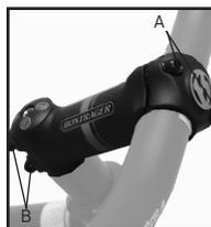
Figure 11- Direct-connect stem
